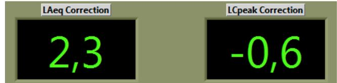
This reflects the difference in the level between what is actually measured by 10EaZy, and what 10EaZy would measure if it were located at the reference point. In the same manner the C-weighted value is subtracted 0.6 dB, as the bass build up under the balcony, makes the C-weighted values higher than what would be measured at the reference point in the audience.
