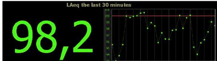
dots on the graph. Every green dot represents a 1-minute average value. The graph is very useful, because it provides the person controlling the sound level with an easy way of knowing if there is “money left in the bank” to increase the average level. The graph will, as a minimum, show 15 minutes of history, i.e. if the Leq period is set to 3 minutes, there will still be 15 dots on the graph.
