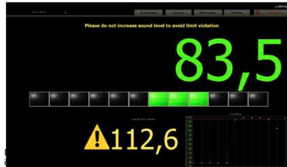
Keeping the sound level below the average level during the period of violation is the only way to get below the limit again, and the period spend over the limit will be directly determined by the sound level at which is played.
