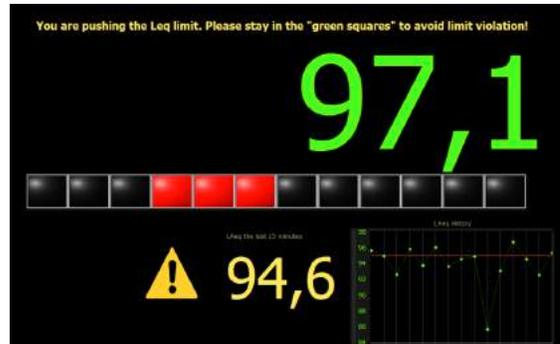
A flashing warning is triggered – Risk of limit violation if level is not reduced to a level where only green squares are lit.
